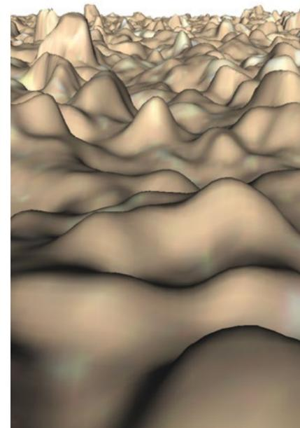
**Surface Level** from Kieran Nar. A focus variation microscopy obtained surface scan of a polymer laser sintered surface
