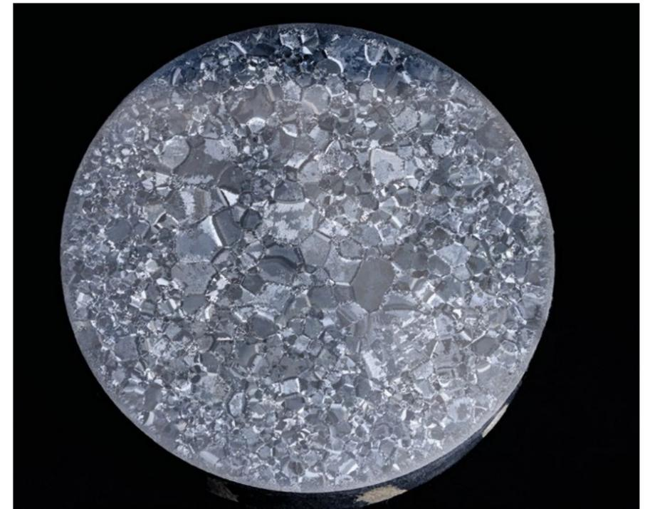
**A Look Beneath the Surface** from Dennis Premoli. A Ti-64 powder 80mm sample, sintered through FAST, polished and etched [courtesy of Rolls Royce]. An attempt at demonstrating the grain growth obtainable through this process and its use is validating new in-process analysis techniques, such as Machining Force Feedback.
