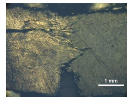
Figure 1. Optical micrograph taken in situ during the fracture of nacre-like graphite showing the action of multiple toughening mechanisms that result in stable crack propagation.
