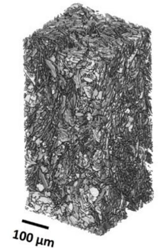
Figure 3. Alignment of microscopic inorganic platelets during processing [in this case hBN platelets in a vitrimer during extrusion] can be analysed using X-ray tomography [in collaboration with the Henry Moseley X-ray Imaging Facility at The University of Manchester]
