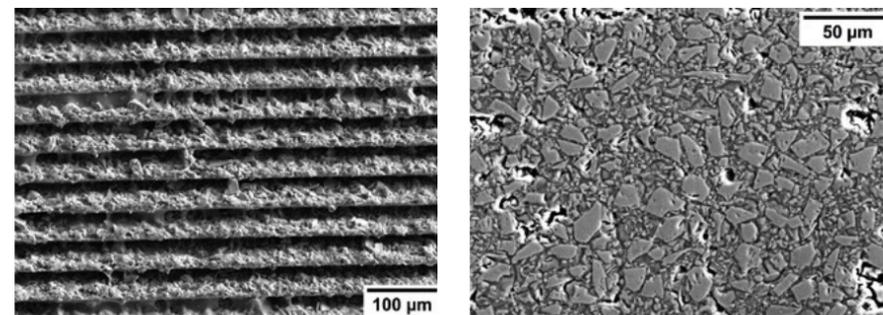
Figure 2. Left, scanning electron micrograph of the surface of a SiC part fabricated using DLP, a characteristic layered surface can be observed. Right, scanning electron micrograph of the microstructure of a SiC part prepared using DLP followed by liquid polymer infiltration pyrolysis. It is possible to densify parts using this process
