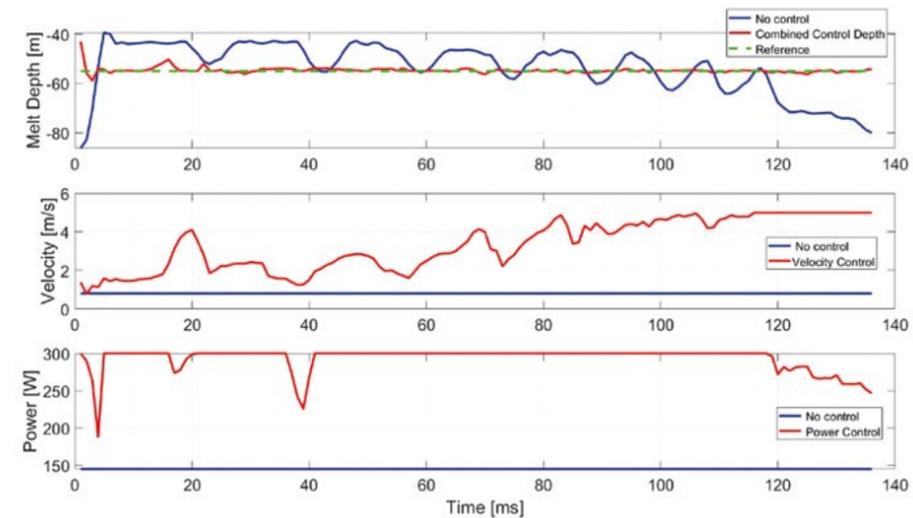
Figure 3. Application of the reinforcement learning, using probabilistic rewards, to the control of the surrogate model.
