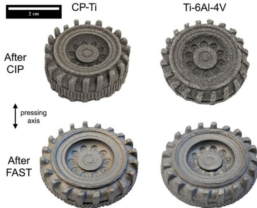
Photographs of CP-Ti and Ti-6Al-4V CIP-FAST parts before and after FAST processing at 980°C for 10 min
