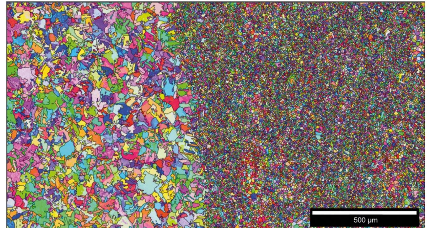
EBSD image of a 2mm x 1mm section of the 0 wt% TiB (left) to 3wt.% TiB (right) interface for a 1400°C 2 hr Ti-6Al-4V sintered sample demonstrating the grain pinning effect of the TiB inclusions
