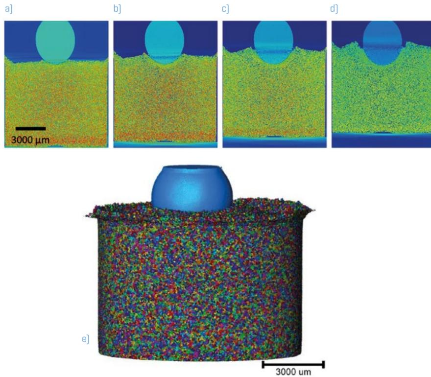
Figure 2: vertical XZ slices of CT images of powders at different indentation depth, (a) 10% (b) 20% (c) 30% (d) 40% scale bar: 3000 μm; (e) 3D volume of particles.
