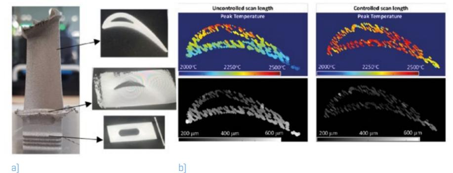
Figure 2. a) Turbine blade built with Controlled scan length and b). Thermal images comparing the two strategies regarding peak temperature and melt pool width
