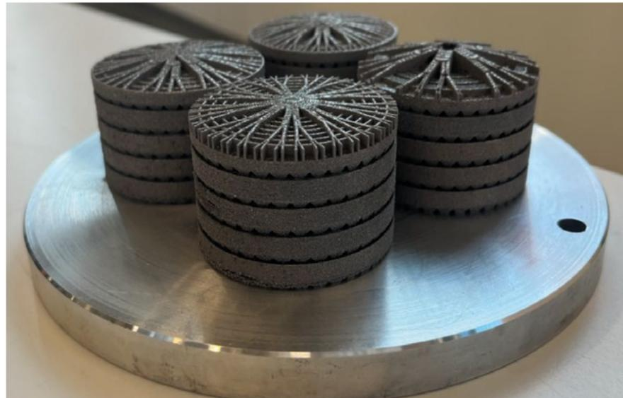
Additively Manufactured aluminium mirrors that are built here as four stacks of five mirrors with different lily-pad lattice designs to reduce the individual component weight. Image courtesy Dr Rob Snell.
