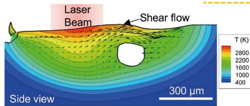
Figure 1. Pore evolution mechanisms in directed energy deposition additive manufacturing revealed with in situ X-ray imaging and multi-physics modelling.
