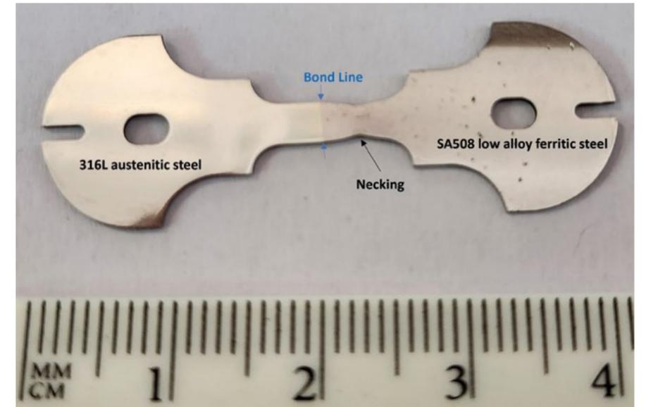
**The Power of Unity: A Dissimilar Joint Stronger Than Its Parent Materials** from Rahul Unnikrishnan. Photo of a tensile test sample of a dissimilar joint between 316L austenitic and SA508 low alloy steel powder processed using FAST tested up to failure. The low alloy steel necked down, demonstrating that the joint is stronger than the parent materials.
