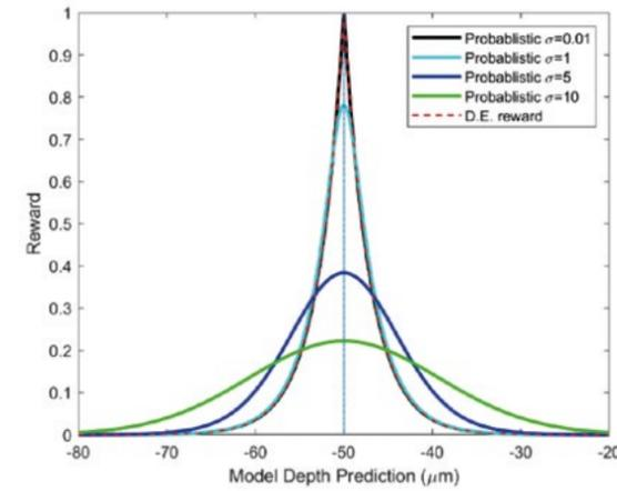
Figure 1. The probabilistic reward function for different levels of prediction uncertainty and a desired target melt pool depth of  $-50\mu\text{m}$ . The scalar reward function is shown as a dotted red line.
