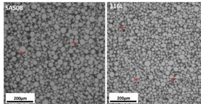
Figure 3 XCT Projection image of SA508 and 316L gas-atomized powders showing internal porosity in the powders (red arrows).
