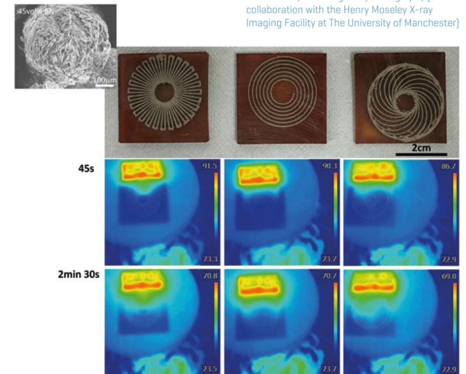
Figure 2. Alignment of hBN platelets during extrusion [inset] combined with direct ink writing enables the printing of materials structures designed to direct heat propagation (from a heat source placed on their side in this example).
