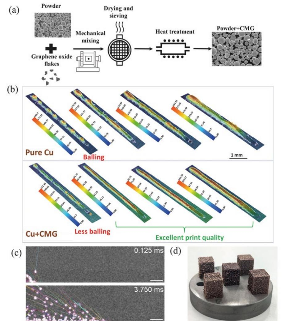
Figure 1. (a) Copper-CMG powder blend preparation. (b) Height map of single tracks for pure copper and Cu+CMG blend showing the improved surface finish and printability with the addition of chemically modified graphene (CMG). (c) Example of in situ process monitoring using synchrotron X-rays where the powder spatter during printing is captured and quantified. (d) Test cubes printed on an industry scale powder bed.
