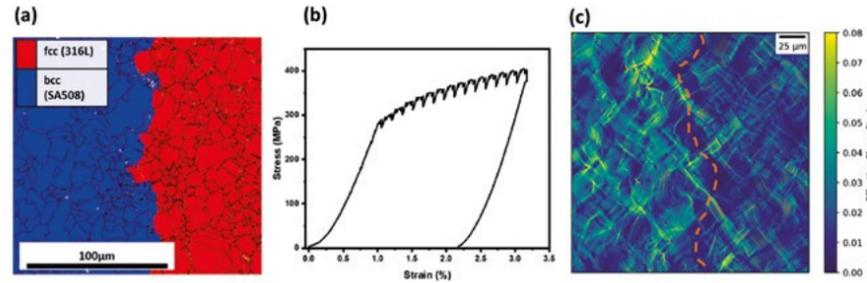
Figure 1 (a) EBSD phase map, (b) Stress-strain curve and (c) 2-D strain maps from digital image correlation of FAST sample (1100°C, 30min dwell, 35 MPa) processed from SA508 and 316L powder. Interface is marked in dashed red lines in (c).
