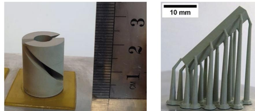
Figure 1. SiC parts fabricated by DLP. The picture on the left shows a small heating element
