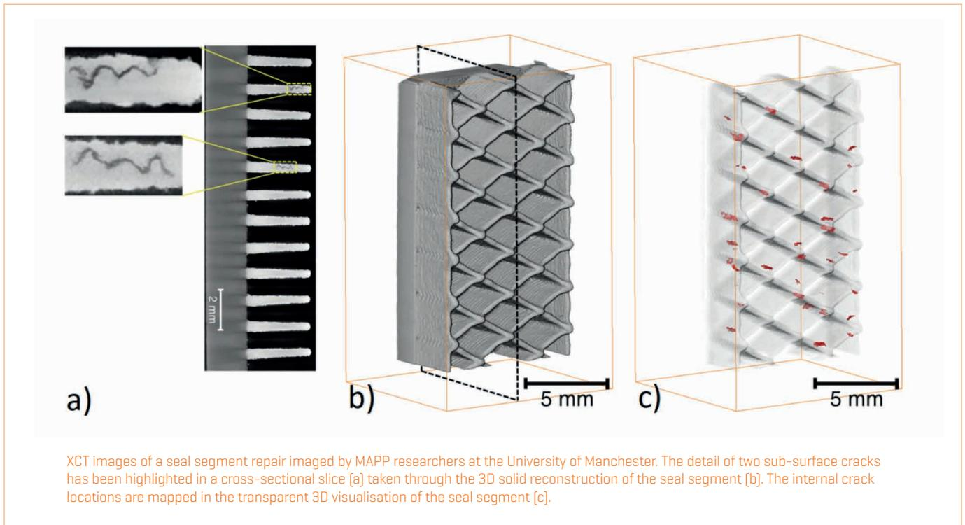
Abradable seals used in Rolls-Royce turbine engine applications are worn down in service and can be subsequently repaired using the blown powder or Directed Energy Deposition (DED) processes.
