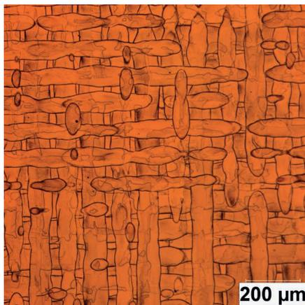
Bidirectional scan tracks in additively manufactured Fe-Si, by Alex Goddall.
