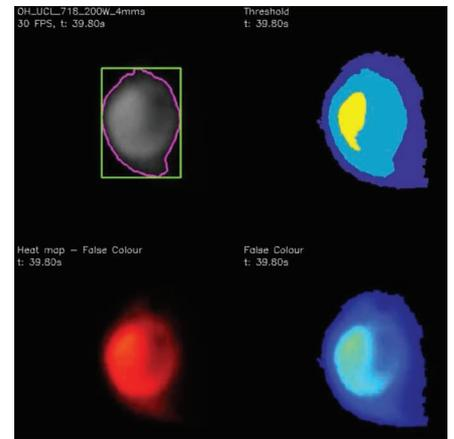
False-colour and heat map images of the melt pool captured *in-situ* during a build using the BeAM machine in Sheffield.
