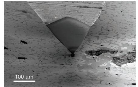
DCB testing of grain boundaries in WC cutting tool. Collaboration SECO tools.
