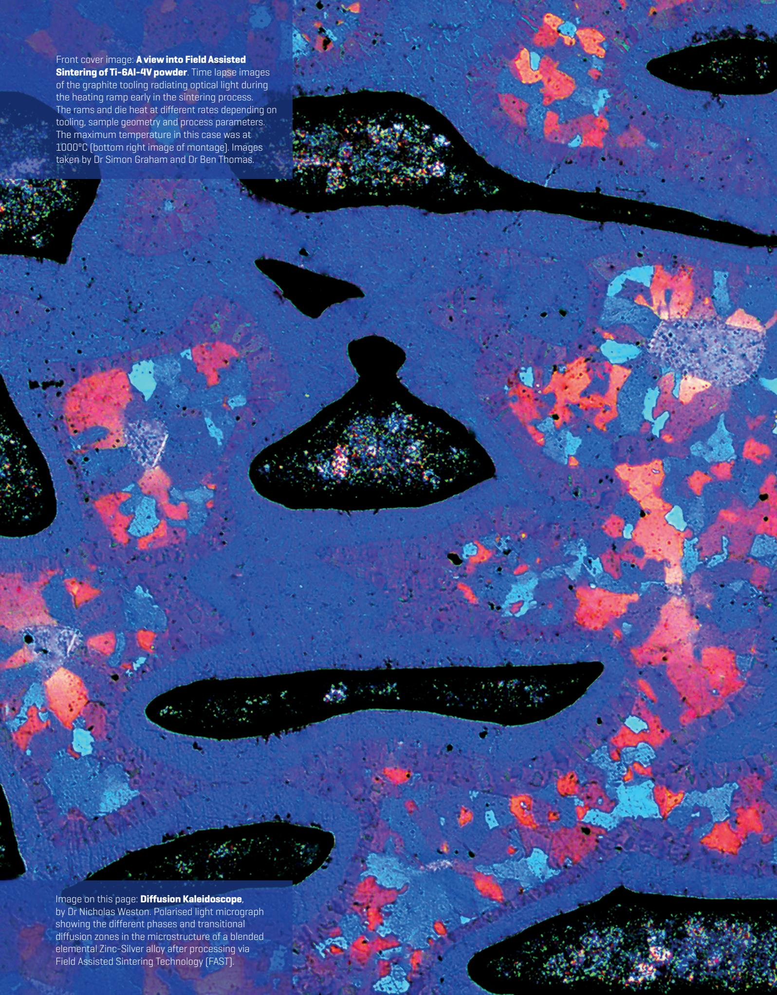
Image on this page: **Diffusion Kaleidoscope,** by Dr Nicholas Weston. Polarised light micrograph showing the different phases and transitional diffusion zones in the microstructure of a blended elemental Zinc-Silver alloy after processing via Field Assisted Sintering Technology (FAST).
