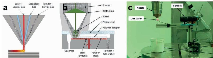
a) BeAM Magic 2.0 nozzle schematic; b) Medicoat AG disc hopper schematic; c) Set-up for side-view flow imaging using line laser.
