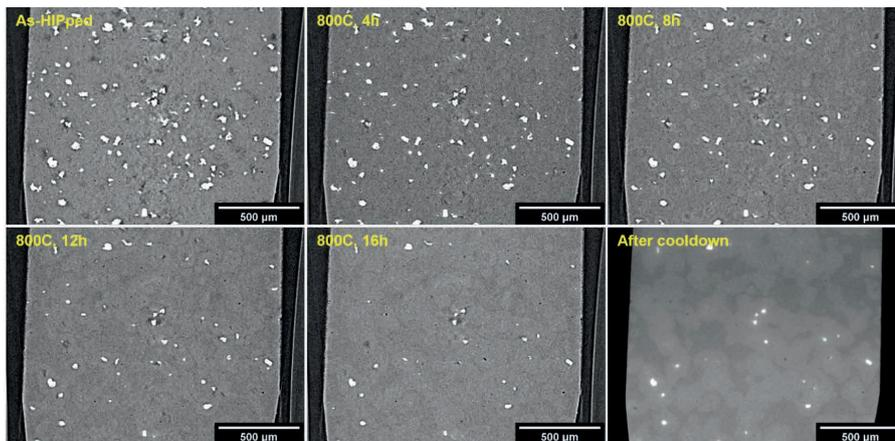
XCT virtual slices showing the same cross-section of an as-HIPed Ti-5 weight %Fe composite during the post-HIPing homogenisation process.
