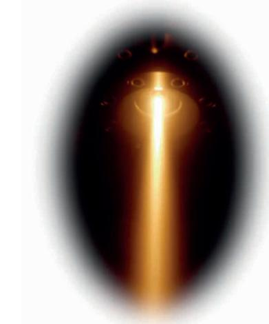
VIGA melt stream atomisation by close coupled die.
