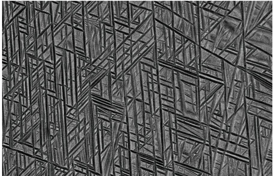
High resolution of geometric perfection by Caterina Iantaffi. A typical basket wave-like microstructure of Ti6Al4V, also called Widmanstätten microstructure.
