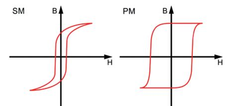
Characteristic magnetic hysteresis loops from a "soft" ferromagnetic material (left) and a "hard" ferromagnetic material (right).
