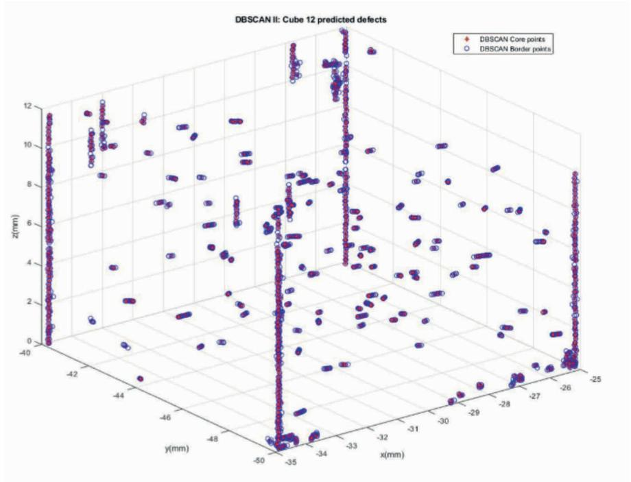
*In-situ* predicted [and XCT validated] part defects [aluminium, LPBF spectral emissions].
