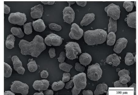
Zhu, Z., et al. [2020] Characterisation and correlation of areal surface texture with processing parameters and porosity of High Speed Sintered parts. *Additive Manufacturing*, **36**, 101402. Micrograph of the virgin PA2200 powders used in this study. Published under Creative Commons CC-BY license. <https://creativecommons.org/licenses/by/4.0/legalcode>.
