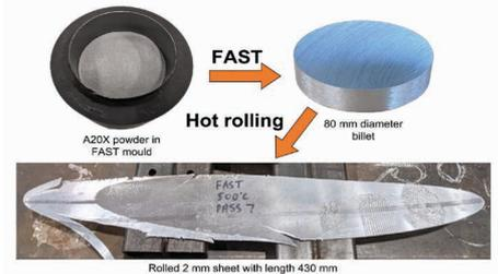
Processing of FAST consolidation combined with hot rolling to convert aluminum alloy powders into sheet product.
