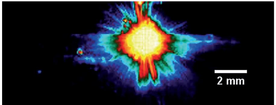
Spattering phenomenon of AISi10Mg during DED-AM process taken by an infrared camera (FLIR X6900SC, US). By Xianqiang Fan.
