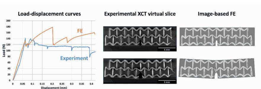
*In-situ* study and modelling on the fracture property of an AM steel-reinforced  $\text{Al}_2\text{O}_3$  matrix composite.
