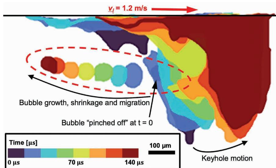
The synchrotron captured the ultra-fast dynamics of keyhole pore formation. Courtesy Yuze Huang.
