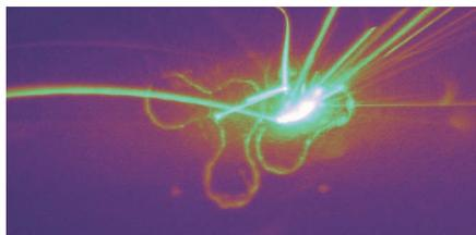
Nickel powder being sintered in a Renishaw Selective Laser Melting machine.
