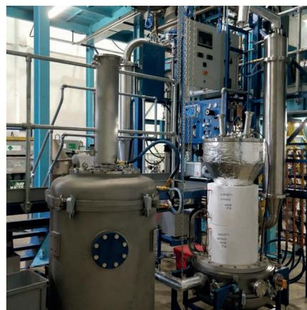
PSI in-house pilot scale Fluidised Bed Reactor for the modification of powders.
