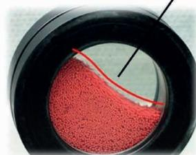
**Example:** Characterisation of DEM particle friction, restitution and cohesion against a GranuTools GranuDrum™ imaged free surface shape
