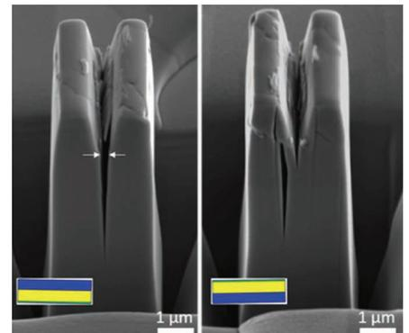
Microscopic Crack propagation in MAX phases.
