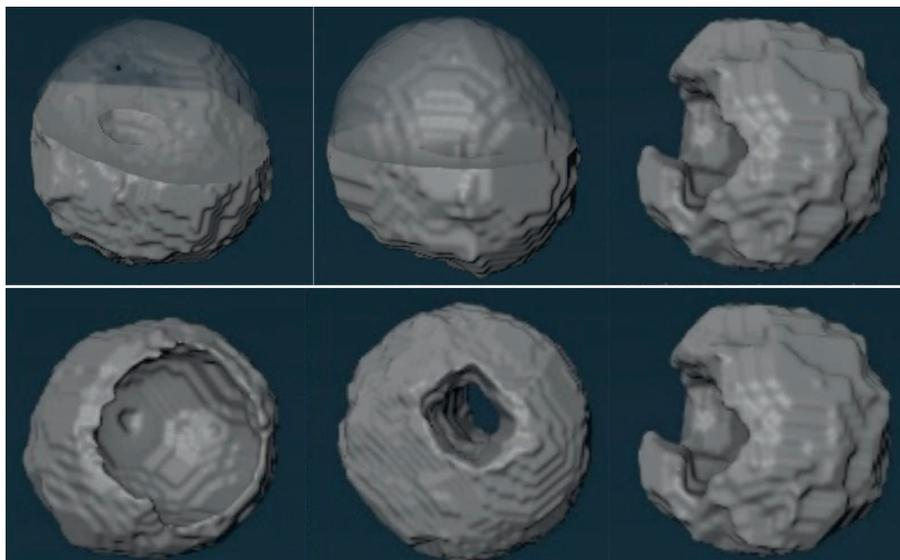
Illustration of hollow and concave particles [gas atomized Ti6] by using X-ray technique.
