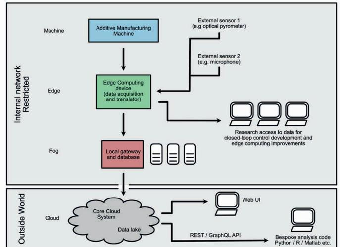
Schematic of the hardware infrastructure to automate complex research data acquisition and management for additive manufacturing.
