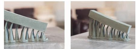
SiC bars prepared by Digital Light Processing: effect of warping.
