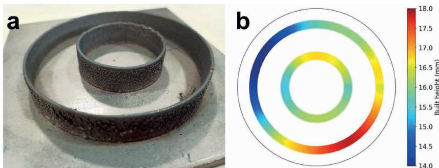
Cylinders built to test whether turntable-frequency flow variation was observable in the physical build. a) Physical appearance of built cylinders; b) Colour map of cylinder height.
