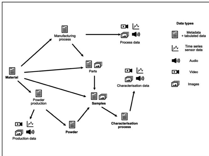
Pseudo data flow chart for a portion of the 'Materials Curation System'. Types of data are shown for each node in the chart.
