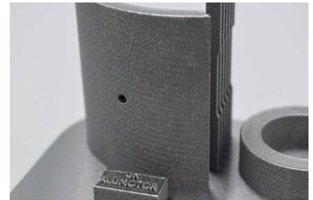
Additively manufactured parts from the Alumotor Project made from a soft magnetic powder developed and manufactured at PSI.
