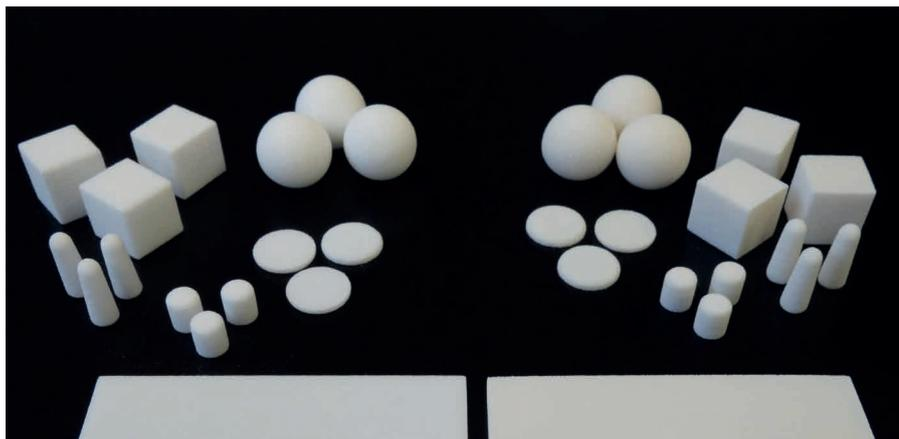
Photograph of a selection of parts made from PA2200 (left) alongside the 1% B65003 composite material (right). Turner, R.D., *et al.* [2019]. Use of silver-based additives for the development of antibacterial functionality in Laser Sintered polyamide 12 parts. *Scientific Reports*. **10**, 892. Creative Commons Attribution 4.0 International License. <https://creativecommons.org/licenses/by/4.0/legalcode>
