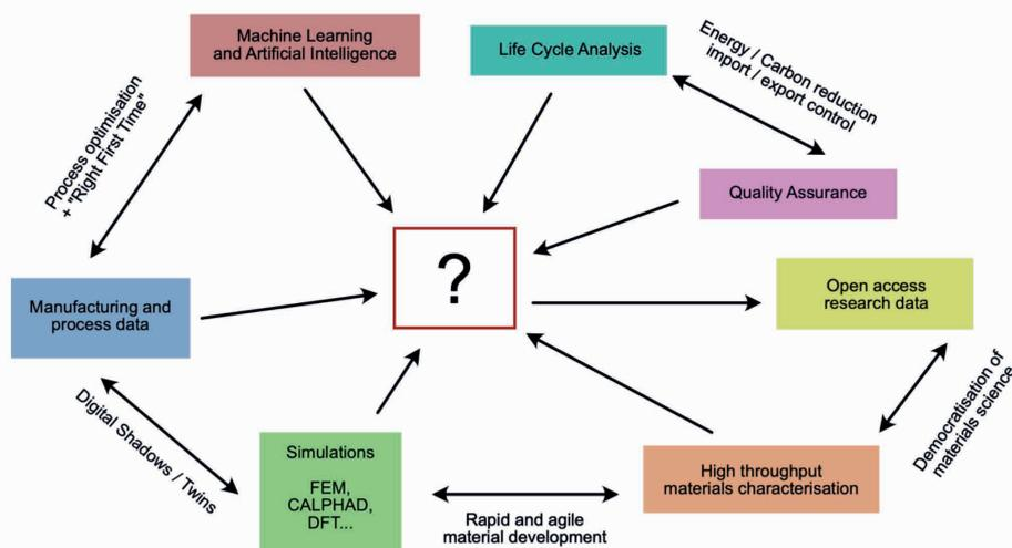
Hub and spoke links between the systems that currently benefit from the digitisation of materials science. Links around the rim of the 'wheel' show some of the areas of "Materials 4.0" under active investigation. The 'hub' that binds all of these systems together, enabling data interchange, still doesn't exist.
