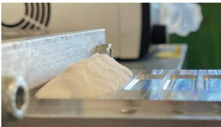
Characterisation of packing density variation during the spreading process using the spreading test rig.
