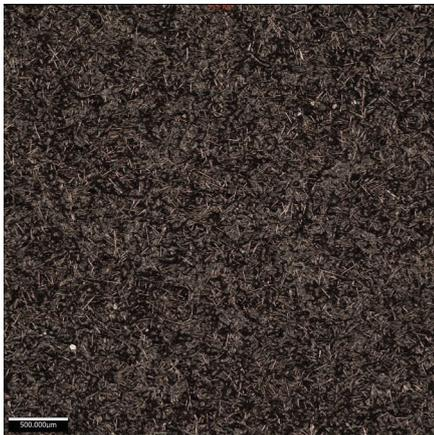
High resolution image of the surface of a carbon-filled polyamide part produced using polymer Laser Sintering. Individual carbon fibres can be seen throughout the base polymer part. Image produced by PhD student Kieran Nar, whose PhD is focused around tribological characteristics of polymer additive manufactured parts.
