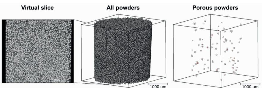
An example showing the XCT image of one powder and individual particles analysed by the automatic workflow. Porous powders are also picked out and highlighted.
