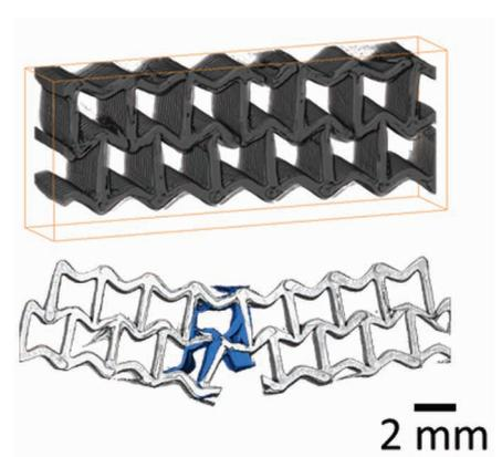
X-ray tomography of a steel auxetic structure embedded in a ceramic ( $Al_2O_3$  in the top) and crack propagation inside the composite (bottom). In collaboration with the University of Manchester.
