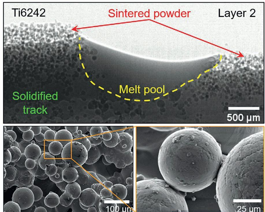
X-ray radiograph image of the melt pool in DED using Ti-6Al-2Sn-4Zr-2Mo alloy, showing a build-up of sintered powder on the track, and SEM images of the powder showing classic sintering necks between particles.
