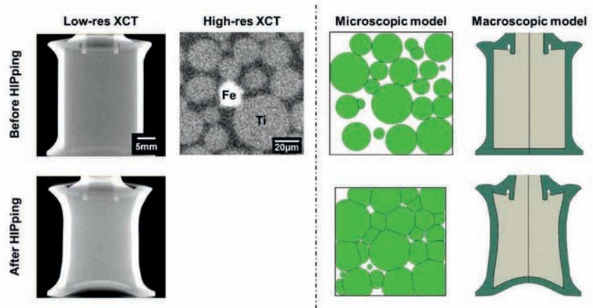
XCT slices [LHS] and microstructurally cognisant models [RHS] showing the sample before and after HIPing on the component [macroscopic] and particle [microscopic] scales.
