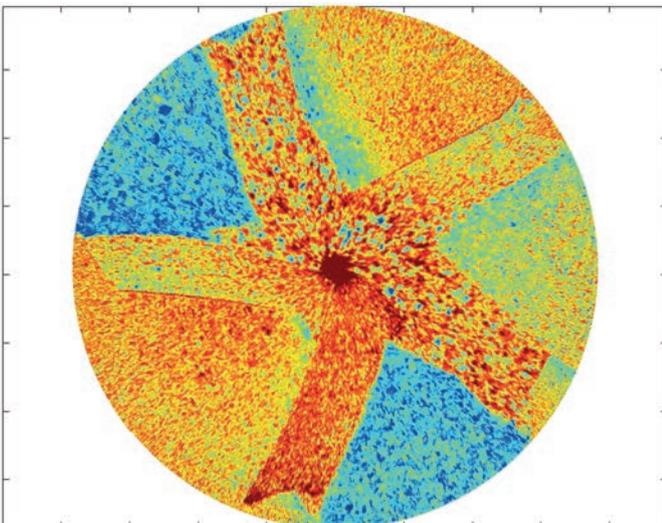
Artefacts and their manufacture runner up image by Dr Oliver Levano Blanch / Dr Daniel Suárez Fernández. This diagram is constructed with the information contained in the forces recorded with a dynamometer during a face turning operation. The machined sample has six different titanium alloys joined by the FAST technology. The alloys are distributed in the shape of the Sheffield Titanium Alloy Research (STAR) group logo.
