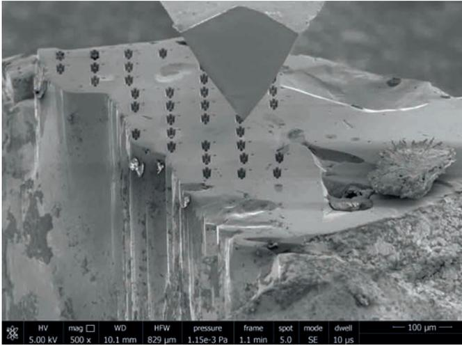
Materials up close winner Max Emmanuel's image showing double cantilever beams (DCB) on the surface of a WC single crystal.
