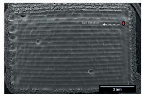
Figure 4 – Top view of laser processed Ti64 using x5 808nm lasers in linear array [3.5W each] simultaneously processing during parallel scans
