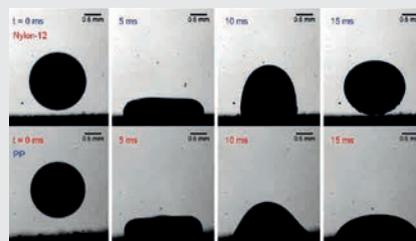
Droplets of identical ink on different polymer surfaces, showing substantial differences in spreading behaviour. Work performed in collaboration with the MAPP team at the University of Leeds.
