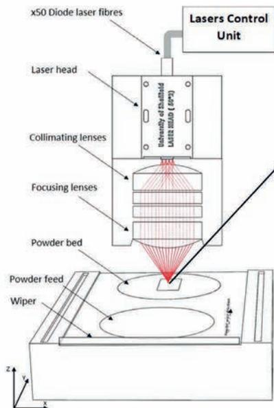
Figure 1 – Diode area melting
