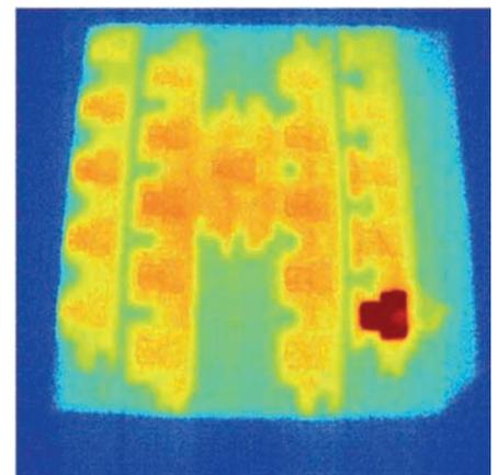
T shaped test pieces showing the effect of residual heat from the previous layer. Boone, N., et al. [2018]. Thermal near infrared monitoring system for electron beam melting with emissivity tracking. *Additive Manufacturing*. **22**, 601-605, Creative Commons CC-BY license. <https://creativecommons.org/licenses/by/4.0/legalcode>.
