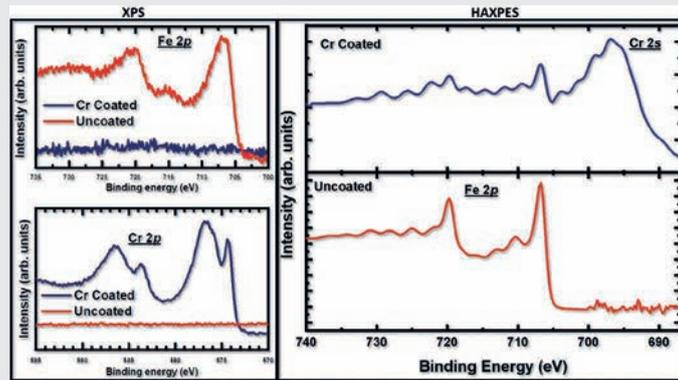
XPS and HAXPES spectrum of Iron and Chromium on uncoated and chromium coated SA508 steel powder. No Iron was detected in XPS spectrum of coated sample whereas HAXPES picked Iron signals on a coated sample.
