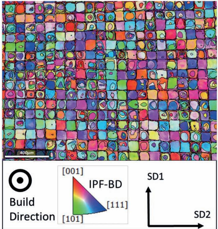
'Assessing the printability of alloys for fusion-based additive manufacturing by coupling thermodynamics phase diagrams and machine learning.' Electron Backscattered Diffraction (EBSD) map of 3D printed alloy that exhibits very low susceptibility to solidification. Inverse pole figure orientation triangle is coloured along the Build Direction (BD). Scanning directions are marked as SD1 and SD2, indicating a 90° rotation between layers. Image by Bogdan Dovggy.
