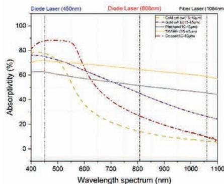
Figure 3 – Increase in absorption at different laser wavelengths
