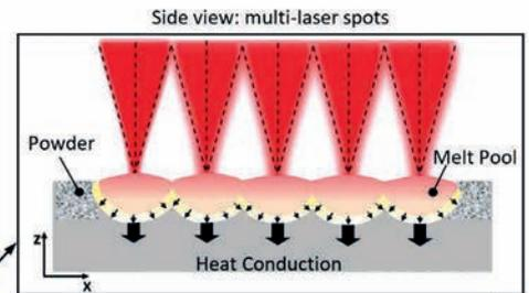
Figure 2 – Individual laser spots and melt pools created on powder bed
