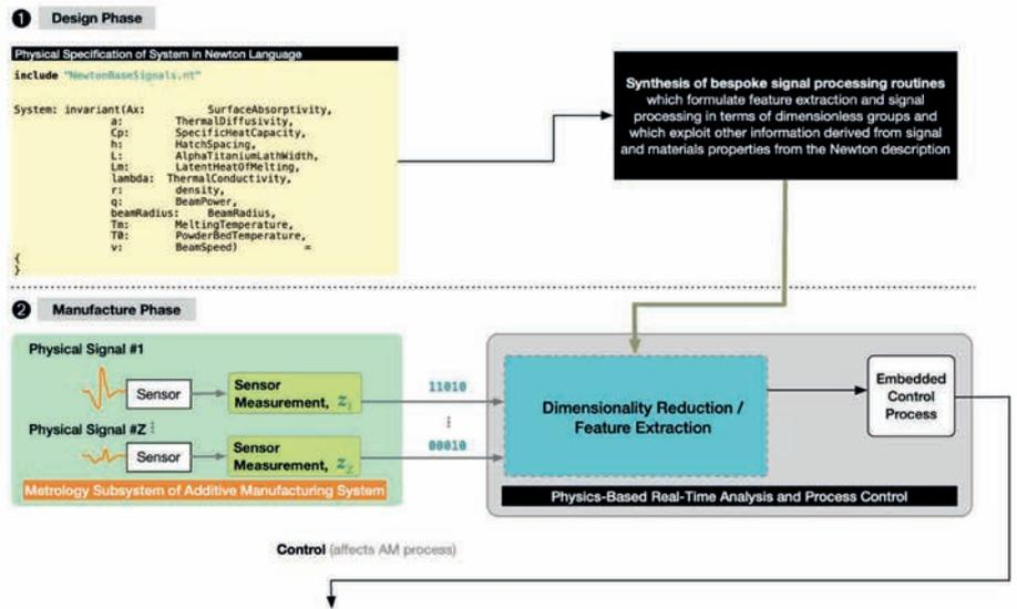
Schematic view of the planned investigation to combine information about physics of materials and manufacture processes to enable new metrology data processing methods where the underlying computational operations exploit knowledge of the physics governing the sources of data they operate on.
